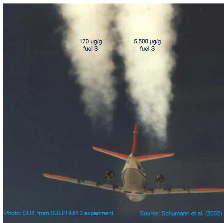
Figure 4-2 Effect of FSC on contrail formation (reproduced with kind permission of DLR)
