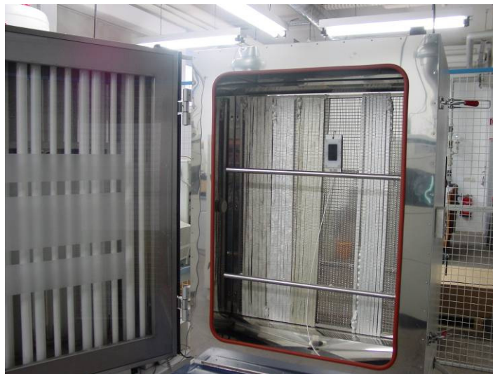
Figure 2: UV-Chamber at STF I – simulation of climate
