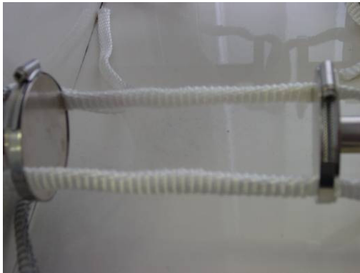
Figure 8: Crushing and torsion test – basic position (STFI e.V.) [11]
