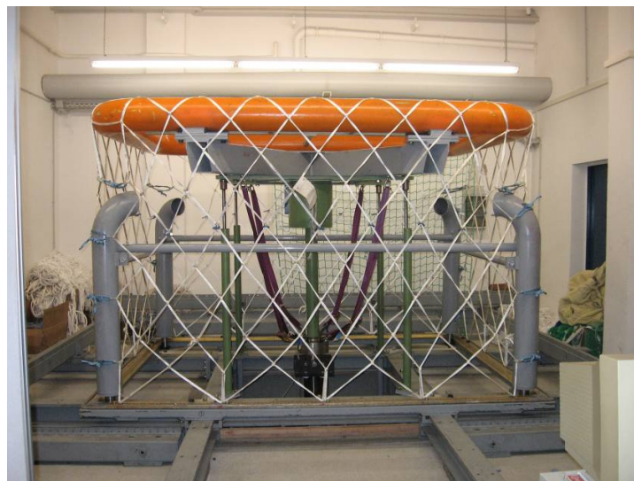
Figure 12: Test set-up for air cargo nets (size 96"x125"x118") at STFI e.V., (full scale test)
